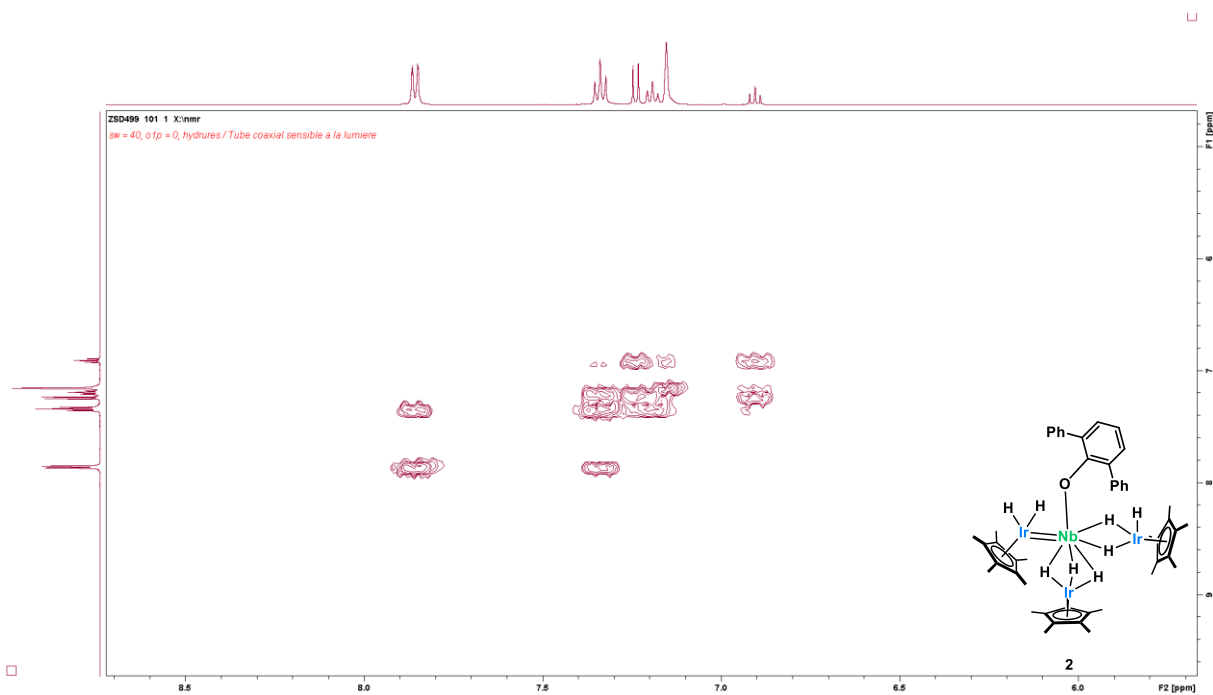
Figure S 10 : 1 H- 1 H COSY NMR spectrum of compound 2 in C 6 D 6 (298K, 500 MHz). Spectra represented along direct and indirect axes are external projections of the 1D spectrum collected on the same sample.
