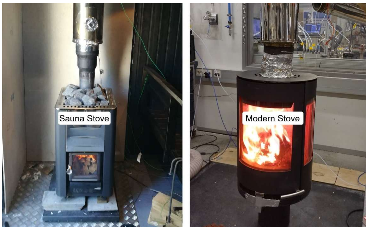
Fig. S1 Photographs of the traditional wood sauna stove (SS) and modern wood stove (MS) tested in the present study.
