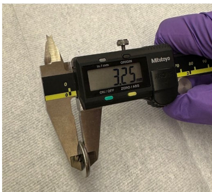
Fig.S5. The thickness of a Zn||Cu half-cell after 50 cycles.
