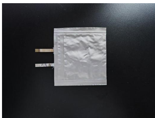
Figure S26. The image of LFP|PHMS|Li pouch cell.
