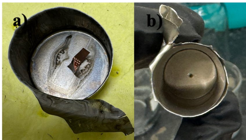
Fig S4. Volume of Electrolyte compared in Fresh cells: a) LIBs with no excess electrolyte, b) NIBs(Hakadi) with excess quantity.
