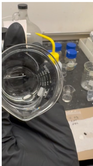
Fig S5. Demonstration of Sodium Metal on Hard Carbon reacting upon immersion in water.
