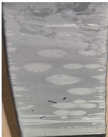
Fig S12. Sodium metal deposition observed on hard carbon negative electrode of Hakadi after testing for 5 cycles at -20^{\circ}\text{C} .
