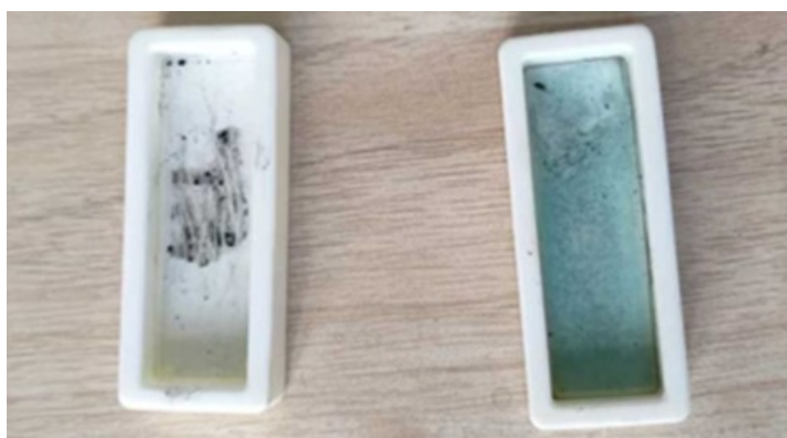
Fig. S8. Image of the alumina crucible surface post- calcination materials in a tube furnace: Tu-333 (Right) and Tu-NCP@333 (Left).
