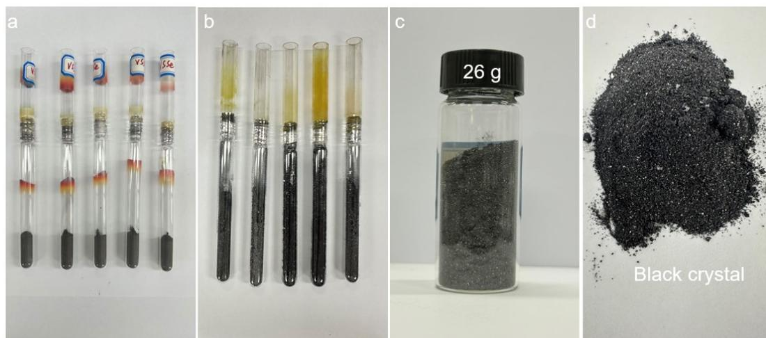
**Figure S2.** The batch preparation of VSSe via PVT method. a) The mixture of V, S and Se powder sealed in vacuum tube, b-d) The obtain product after annealing.
