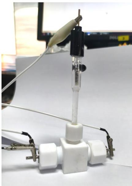
**Figure S5.** A three-electrode Swagelok cell with a Hg/HgCl<sub>2</sub> reference electrode.
