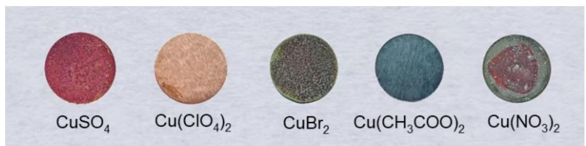
**Fig. S17** Optical images of Cu foils immersed in different electrolytes for 5 days.
