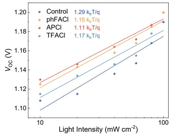
**Fig. S15.**  $V_{OC}$  as a function of light intensities for the control and phFACl, APCI and TFACl modulated PSCs.
