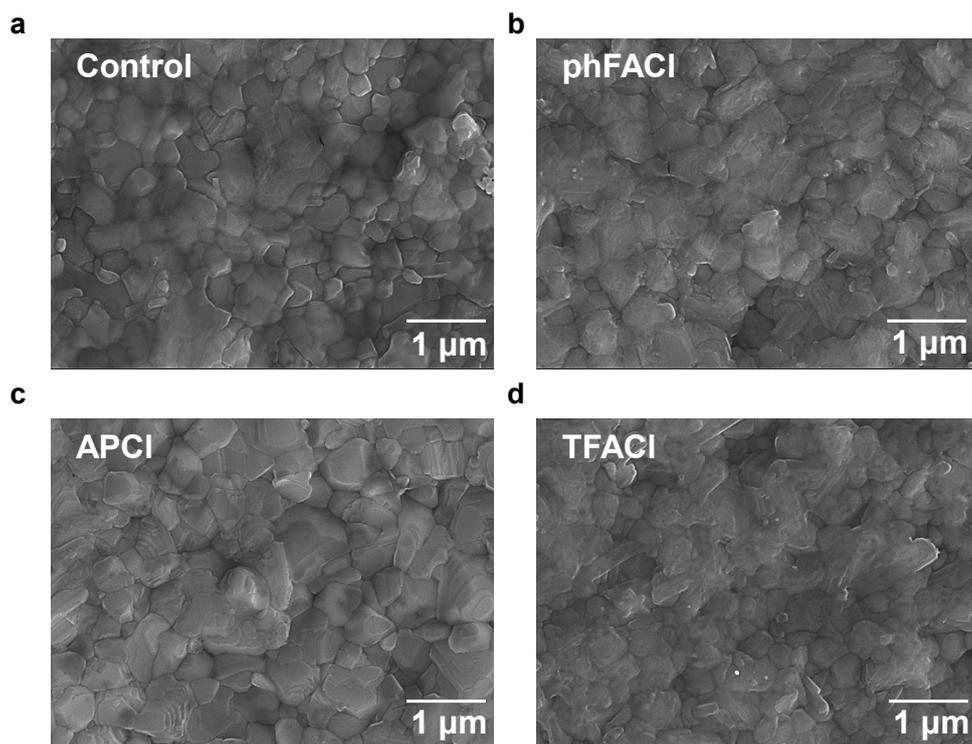
**Fig. S2.** SEM images for the (a) Control, (b) phFACl, (c) APCl and (d) TFACl-modulated perovskite films.
