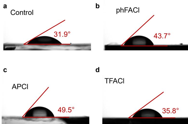
**Fig. S20.** The contact angle of the control, phFACl, APCl, and TFACl-modified perovskite films.
