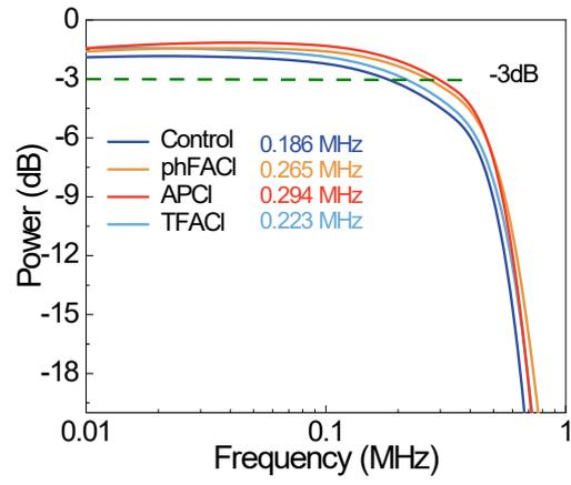
**Fig. S18.** The frequency response of the control and phFACI, APCI and TFACI-modulated devices.
