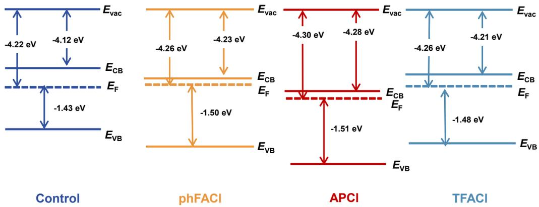
**Fig. S4.** Energy-level diagram of the control, pHFACl, APCI, TFACl modulated perovskite films.
