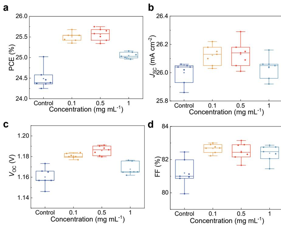
**Fig. S8.** Statistics of  $V_{oc}$ , FF, PCE and  $J_{sc}$  of the PSCs modulated by different concentrations of TFACI. The statistic data were obtained from individual 7 devices for each kind of PSCs.
