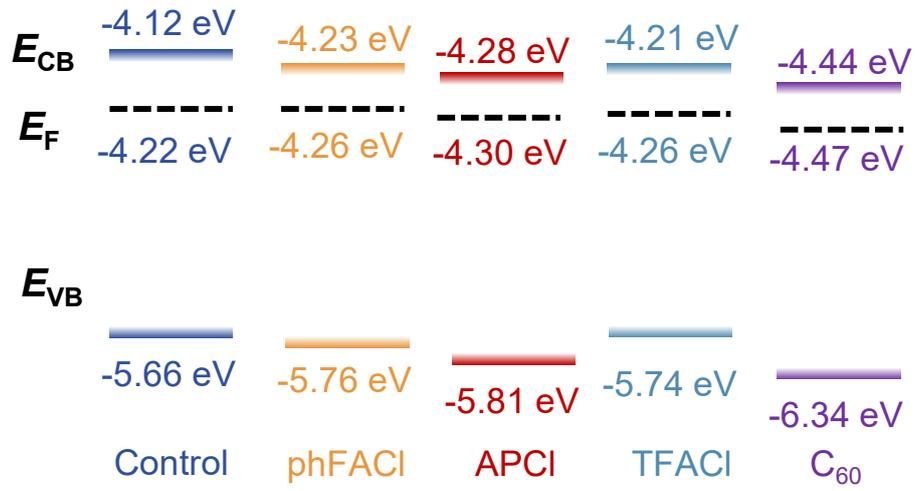
**Fig. S3.** Energy-level diagram of the control, phFACl, APCI, and TFACl modulated perovskite films as well as C<sub>60</sub>.
