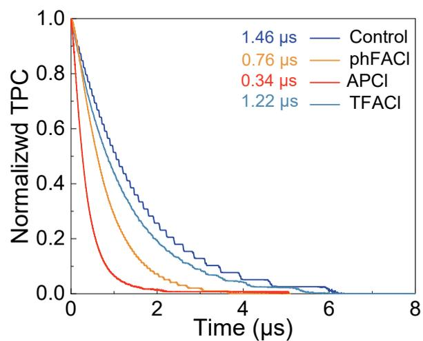
**Fig. S16.** TPC curves for the control and phFACI, APCI and TFACI-modulated devices.
