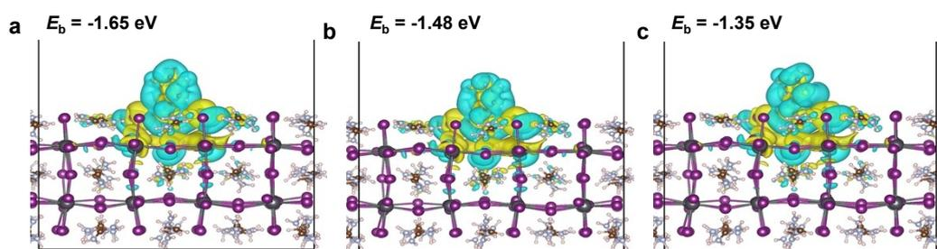
**Fig. S1.** The binding energy of  $\text{phFA}^+$ ,  $\text{AP}^+$ , and  $\text{TFA}^+$  with  $\text{FAPbI}_3$  containing  $\text{V}_I$  and  $\text{V}_{\text{FA}}$  defects in vertical configuration.
