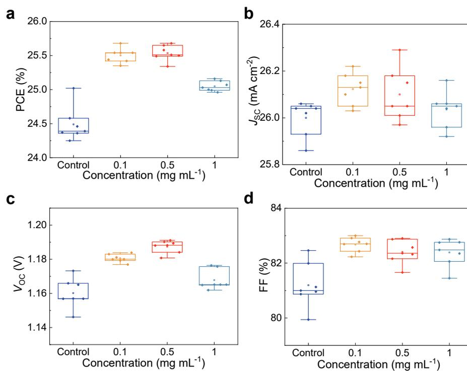
**Fig. S6.** Statistics of  $V_{oc}$ , FF, PCE and  $J_{sc}$  of the PSCs modulated by different concentrations of phFACl. The statistic data were obtained from individual 7 devices for each kind of PSCs.
