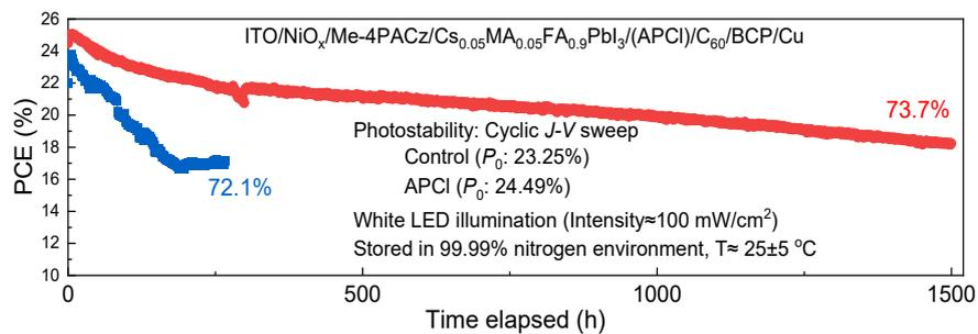
**Fig. S19.** PCE output changing from cyclic  $J$ - $V$  scanning measurement of the control and APCI-modulated PSCs.
