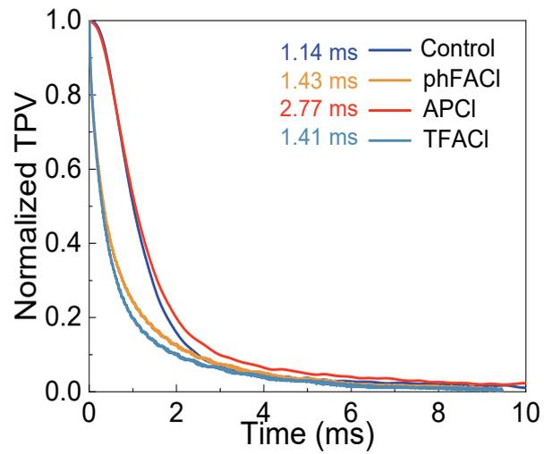
**Fig. S17.** TPV curves for the control and phFACI, APCI and TFACI-modulated devices.
