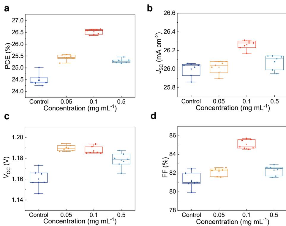
**Fig. S7.** Statistics of  $V_{oc}$ , FF, PCE and  $J_{sc}$  of the PSCs modulated by different concentrations of APCI. The statistic data were obtained from individual 7 devices for each kind of PSCs.
