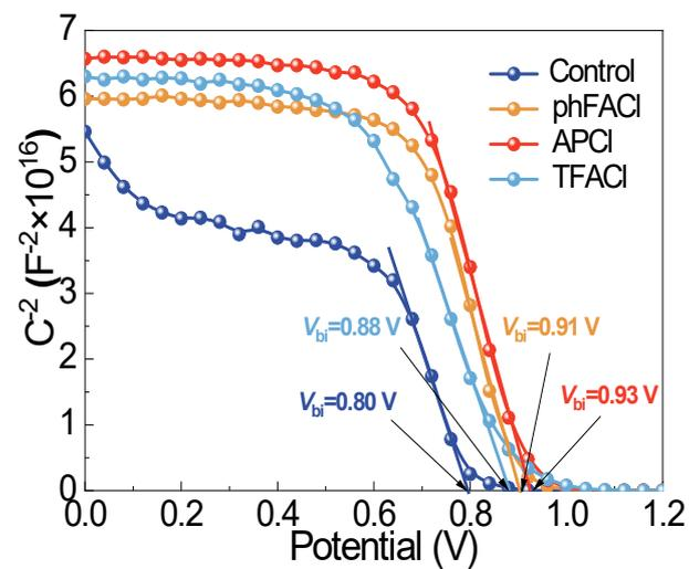
**Fig. S5.** Mott–Schottky plots of the control and phFACl, APCI, TFACl-modulated PSCs.
