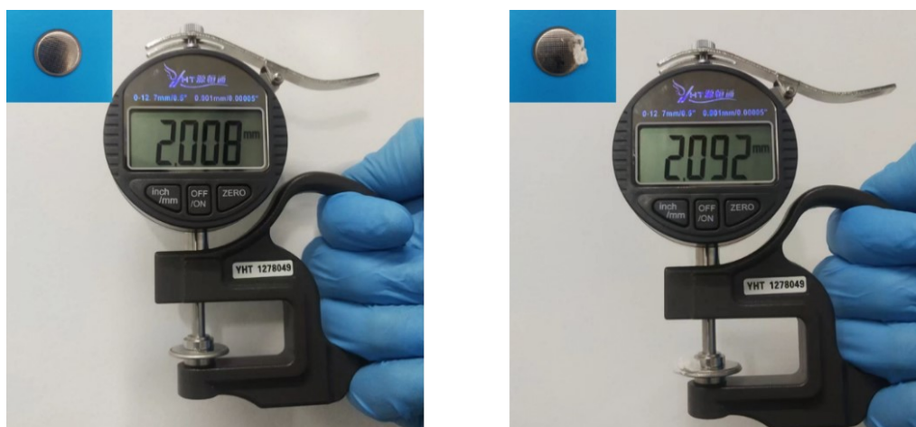
Figure S27. Graphs of the cell thickness results with SDCD@Zn (left) and bare Zn (right) anodes after cycling (Insets show tested cell).
