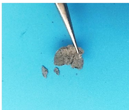
Figure S22. The deposited Zn layer of 10 \text{ mAh cm}^{-2} on bare Ti and SDCD@Ti.
