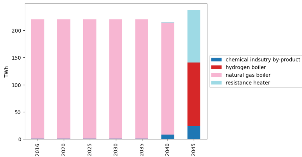
Supplementary Figure 7: High temperature (HT) industrial heat production mix transition pathway. Only 0.5% of HT heat is produced via resistance heaters in 2040. In 2045, all HT heat transitions away from natural gas boilers due to the exogenous net-zero emissions constraint. The late transition of high temperature heat to electrified technologies is driven by the high capital cost assumptions for resistance heaters and hydrogen boilers. Results considering optimistic cost assumptions are presented in Section 5
