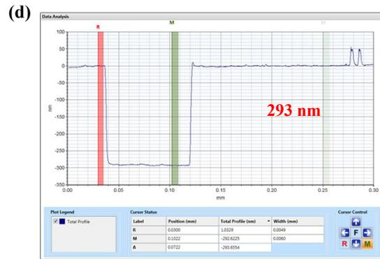
**Supplementary Figure 9.** Thickness results of 147 nm, 205 nm, 253 nm, and 293 nm films from a surface profilometer.
