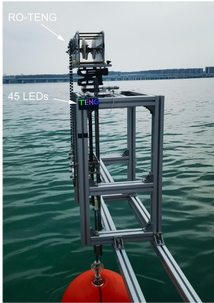
**Fig. S26:** Using the RO-TENG to light up 45 LEDs in the ocean environment.
