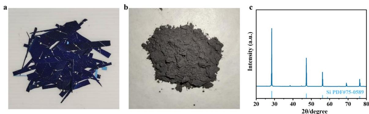
**Figure S1.** Photographs of (a) waste c-Si PV cell fragments, and (b) milled c-Si PV cell powder. Using Dong Yi multi-function pulverizer 800Y, rated power: 1400W, motor speed: 3400r/min, pulverizing time: 5 min. (c) Powder X-ray diffractogram of milled c-Si PV cell powder alongside reference pattern for Si (PDF: 075-0589).
