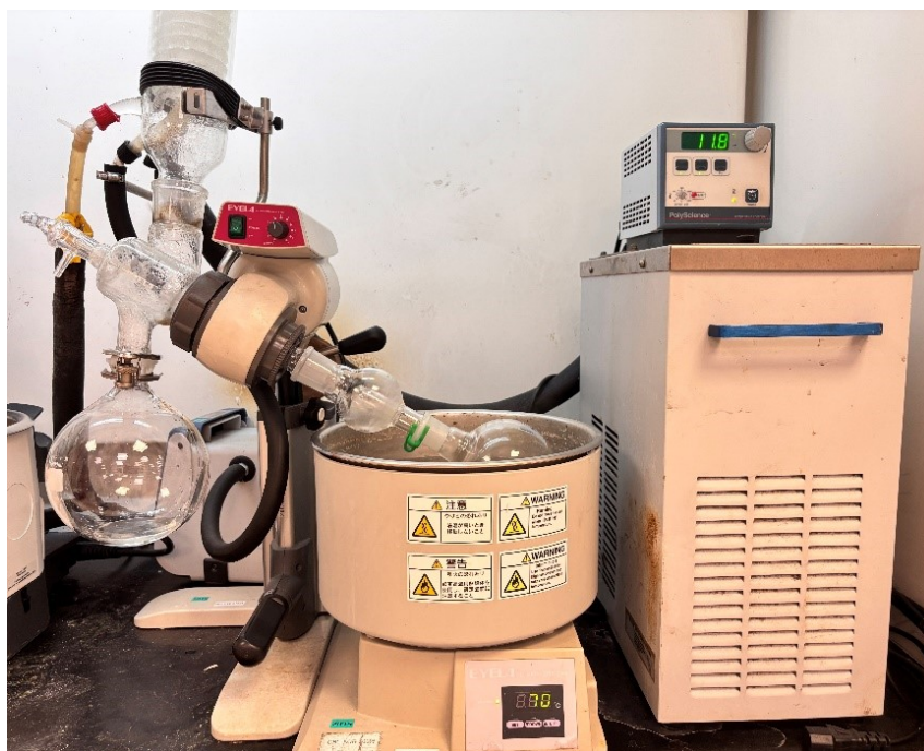
Fig. S54. Photo of the removal of water from the product using a rotary evaporator at 70 °C.
