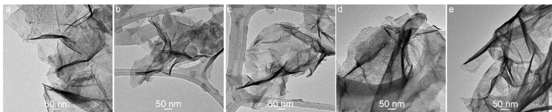
Fig. S2. TEM images of (a) \text{Co(OH)}_2 , (b) \text{Ru-0.2-Co(OH)}_2 , (c) \text{Ru-1-Co(OH)}_2 , (d) \text{Ru-5-Co(OH)}_2 , and (e) \text{Ru-10-Co(OH)}_2 .
