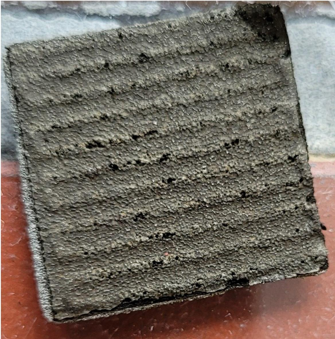
Supplementary Figure 11: **NiFe-LDH@NF anode after 200 h electrolysis.** Morphology change, new layer with cracks on top of the foam.
