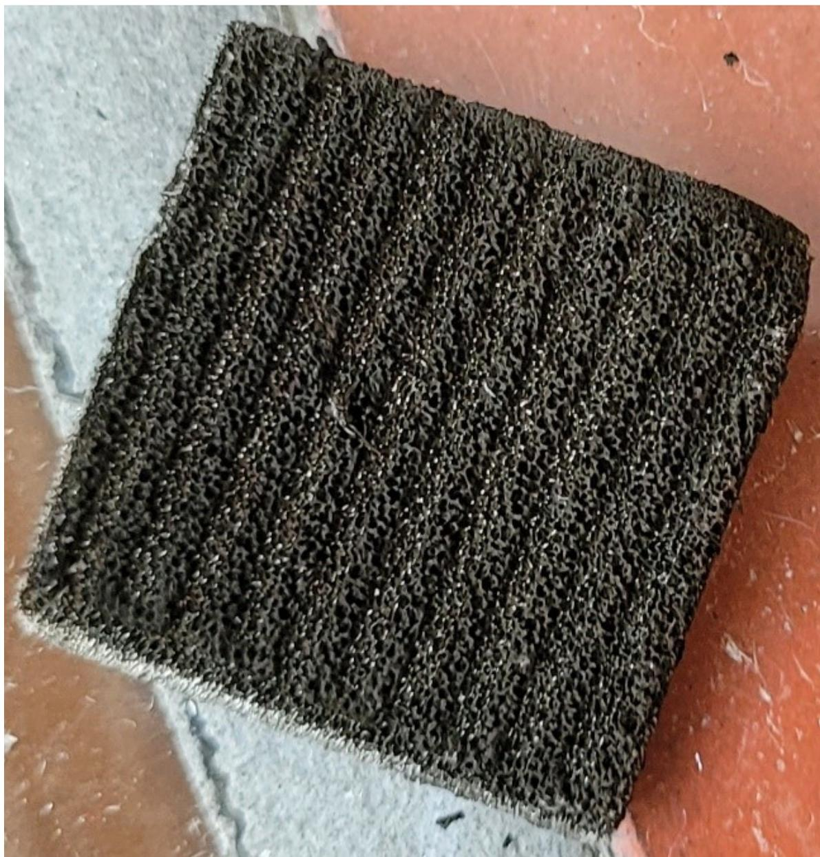
Supplementary Figure 13: **Back side of the Anode with an unchanged foam texture.**
