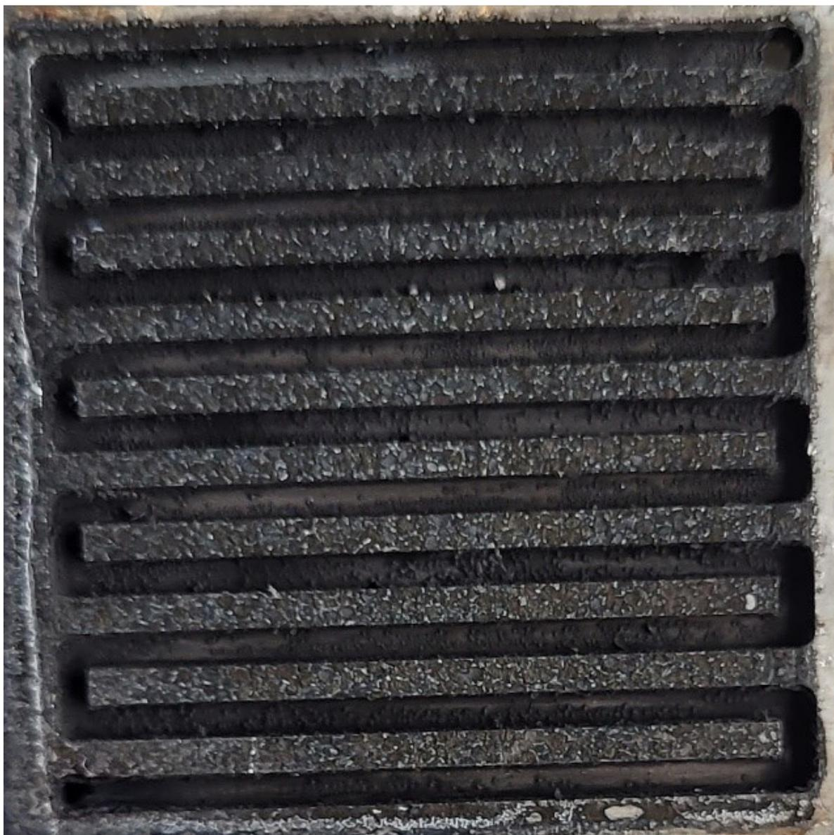
Supplementary Figure 12: **Anode serpentine flow field covered with particles.**
