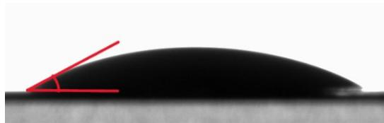
**Fig. S3** Wettability test of the 0.5M-D and 0.5M-FD electrolytes on bare Na.
