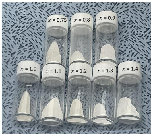
**Supplementary Figure 1.** Photograph of vials containing Li-Al-O-Cl solid electrolytes ( $0.75 \leq x \leq 1.4$ ). All samples exhibit a powder-like morphology, indicating the absence of viscoelastic behavior.
