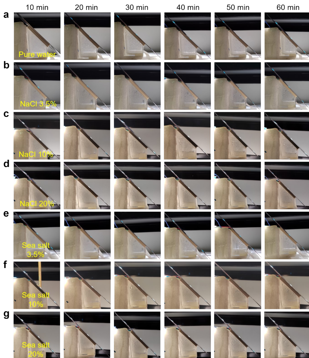
Fig. S21 Water collection situation of A13-ACPGF in salt solutions of different concentrations under 1.0 sun for 1 hour, including time periods of 0, 10, 20, 30, 40, 50, and 60 min. (a) Pure water, (b) NaCl 3.5 wt%, (c) NaCl 10 wt%, (d) NaCl 20 wt%, (e) Sea salt 3.5 wt%, (f) Sea salt 10 wt%, and (g) Sea salt 20 wt%.
