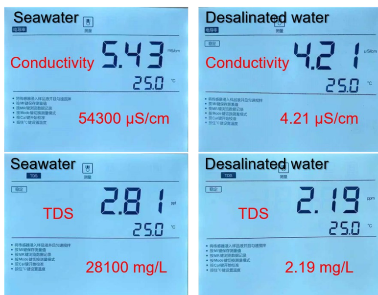
Fig. S13 Comparison of conductivity and TDS measured by Water Quality Tester between 3.5 wt% simulated seawater and the water collected by ACPFG.
