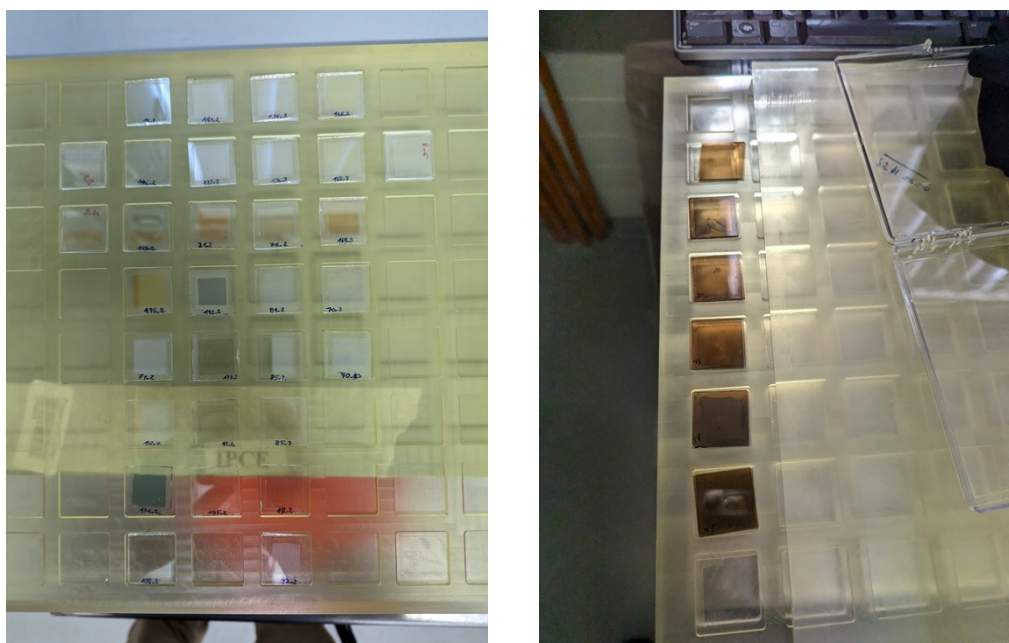
Figure S3: Pictures of samples in the Perspex (PMMA) phantom before (left) and after (right) gamma degradation.
