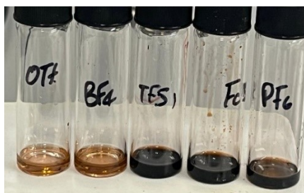
Supplementary Figure S7. Photographs of spiro-OMeTAD solutions in chlorobenzene ( 90 \text{ mg ml}^{-1} ) prepared using ferrocenium doping with different anions from left to right: [\text{Fc}][\text{OTf}] , [\text{Fc}][\text{BF}_4] , [\text{Fc}][\text{TFSI}] , [\text{Fc}][\text{I}_3] , [\text{Fc}][\text{PF}_6] .
