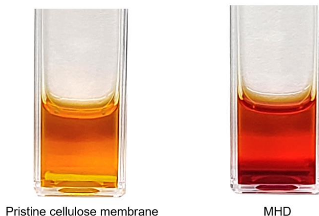
Figure S8. Photographs of the pristine cellulose and the MHD immersed in methyl orange/water solution (0.1% w/v in water). The methyl orange solution is a typical pH indicator, changing from orange to red when the pH changes from 4.4 to 3.1. For the MHD, the solution color changes from orange to red, indicating the presence of acid groups (e.g. sulfuric and sulfonic acid groups) that release abundant H^+ ions upon contact with water. In contrast, pristine cellulose shows limited H^+ dissociated from hydroxyl groups.
