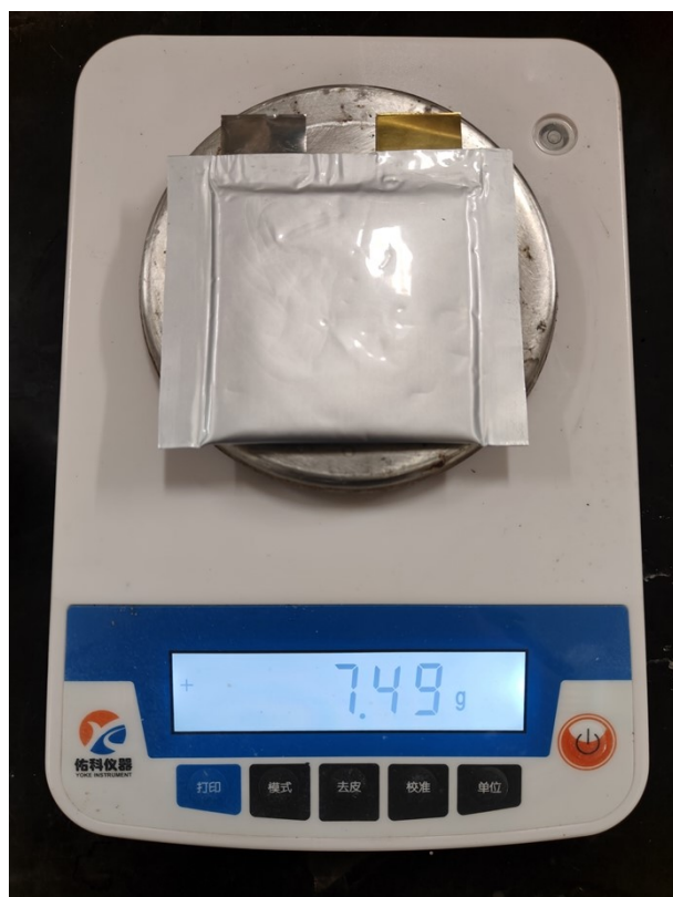
Fig. S38. Digital photo of the Zn-Br 2 pouch cell weighed on an analytical balance.
