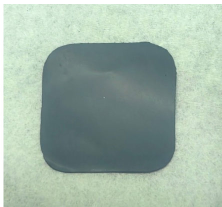
Supplementary Fig. 12 | Composite cathode dry film with 0.2wt% PTFE.
