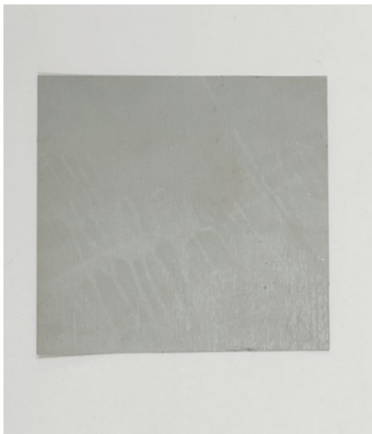
Fig. S41 Digital photograph of Zn plated on a Cu foil at a current density of 6.6 \text{ mA cm}^{-2} in the Ect electrolyte.
