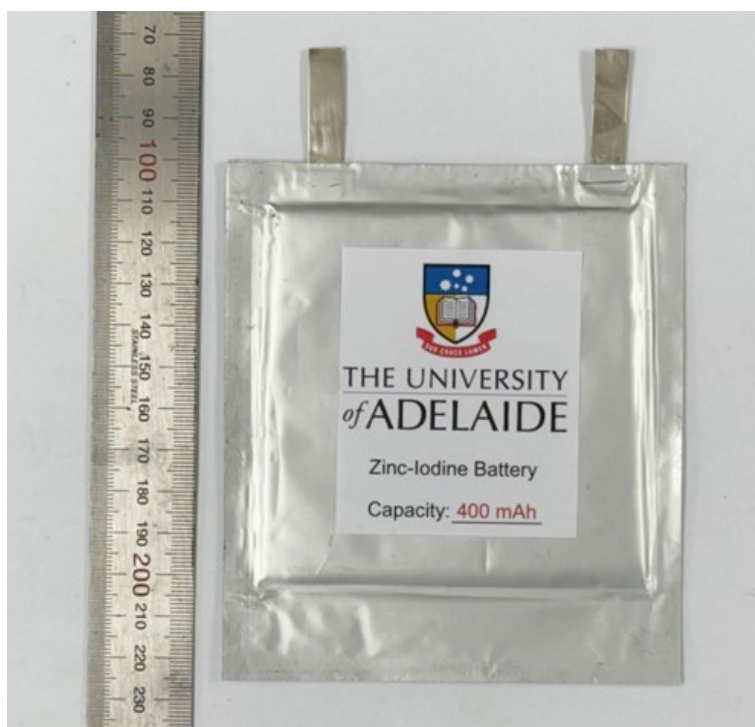
Fig. S39 Digital photograph of the 400 mAh Zn-I 2 pouch cell.
