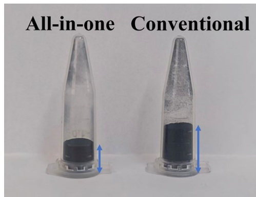
Figure S3 Photograph of S@FG-NP AE materials and S@FG-NP CE materials with the same mass.
