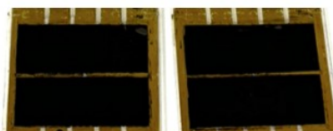
Supplementary Figure 20: Images of pair of PSCs post 200 hours of accelerated ageing under ISOS-L-2 equivalent. (85°C, 0.76 suns illumination, open circuit condition, without UV filter) fabricated under a) 0%RH and b) 35%RH respectively.
