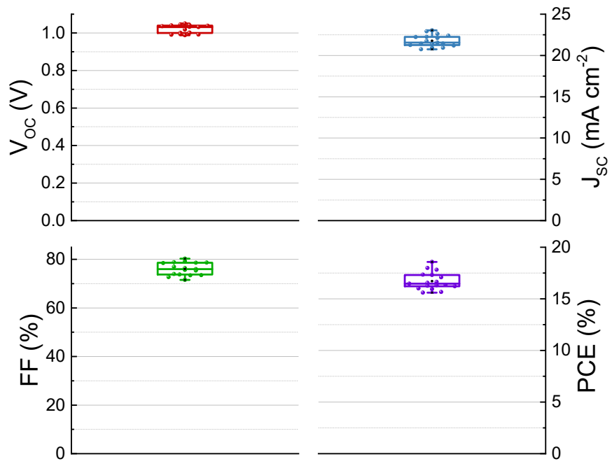
Figure S19: Electrical parameters ( V_{OC} , J_{SC} , FF and PCE) distribution from one batch of Type-300A-based devices.
