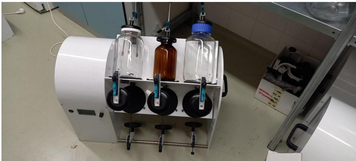
*Figure S3. Overhead Tumbler for textile washing*
