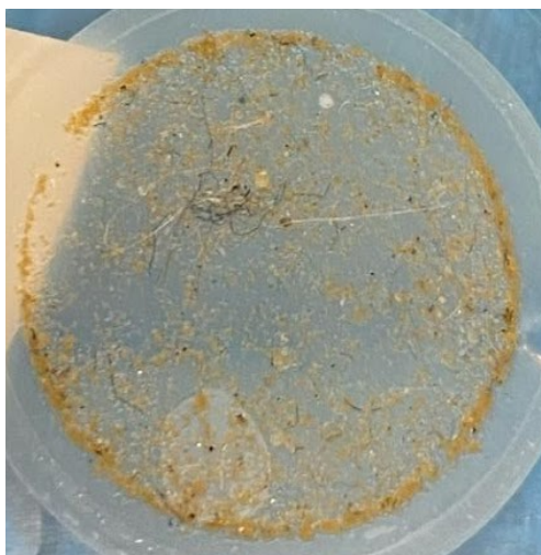
Figure S2. Sample 2, after a 1:1 addition of denatured ethanol to the sample volume (Method 4), was filtered onto an Anodisc analysis filter.
