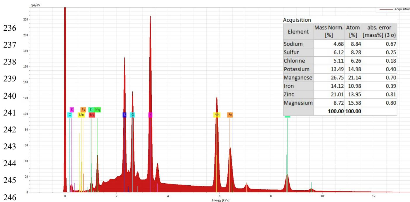
249 **Figure S6.** SEM-EDX elemental profile of the nano-Zn-Mg-Mn-Fe composite showing the
