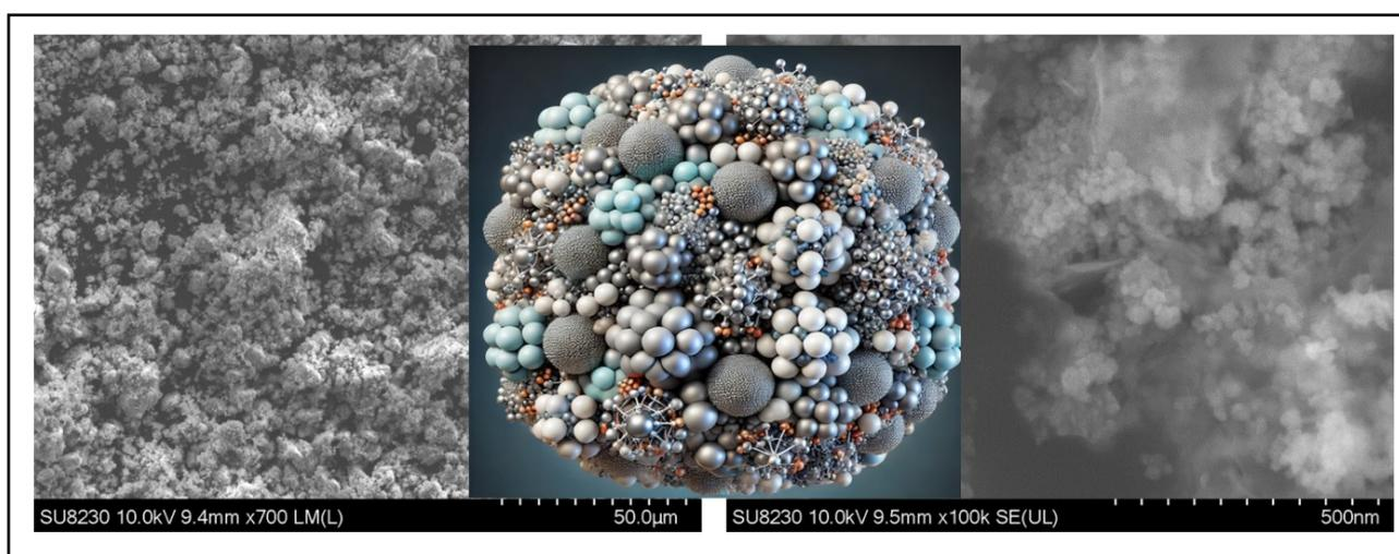
63 **Figure S1.** A detailed representation of the Nano-Zn-Mg-Mn-Fe composite using SEM
