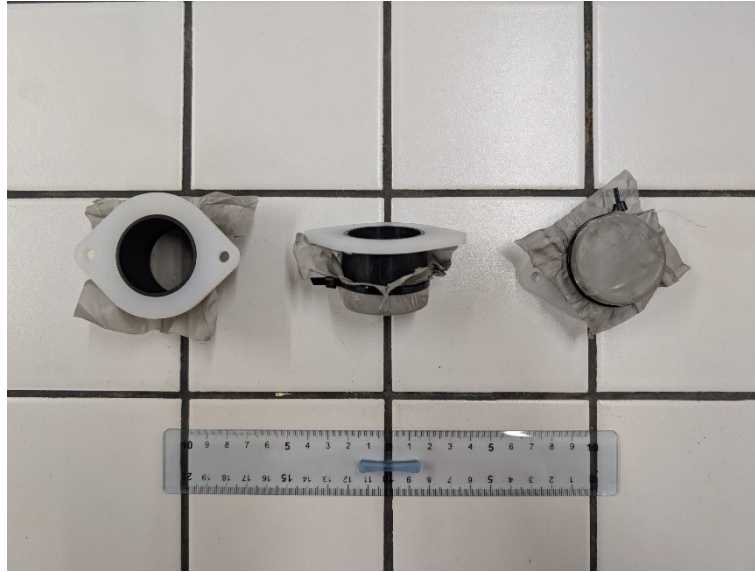
Figure S1. HDPE pots, sealed at the bottom with a 30-μm pore-size stainless steel mesh, were used for the germination, growth and exposure of tomato plants
