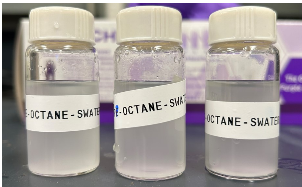
Figure S2: Photographs of emulsions produced from LDPE (left), PP (middle) and PS (right) in artificial sea water in the presence of 1% Octane.
