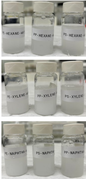
Figure S5: Photographs of emulsions containing mixtures of sMPs and NPs of LDPE, PP, and PS in water produced in the presence of hexanes (top), xylene (middle) and naphtha (bottom).
