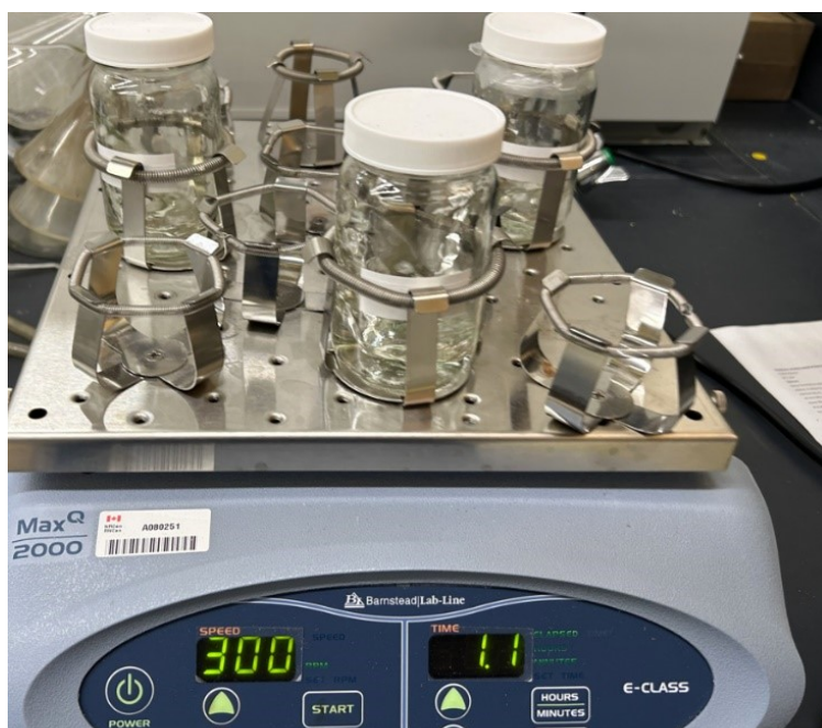
Figure S4: Rotary orbital shaker used for low-energy mixing.
