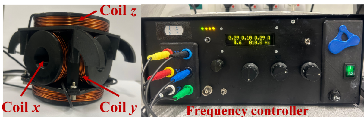
Figure S11. Pictorial images of the custom-built magnetic setup utilised during the experiments.
