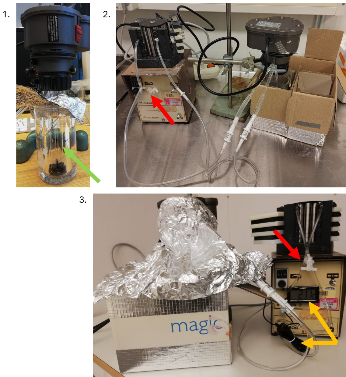
Figure S3. Experimental setup for UVC treatment. Panel 1 shows the UVC lamp submerged in 385 mL of Milli-Q H 2 O (green arrow). Panel 2 depicts the UVC lamp immersed in the liquid and connected via tubing and glass rods to a peristaltic pump for solution circulation. The red arrow indicates the valve used for sample withdrawal during UVC treatment. Panel 3 presents the complete setup. Aluminum foil was used to prevent UVC light from escaping the system. A thermometer, with its sensor taped beneath the aluminum foil to the glass rod guiding the circulating solution out of the beaker, is indicated by orange arrows.
