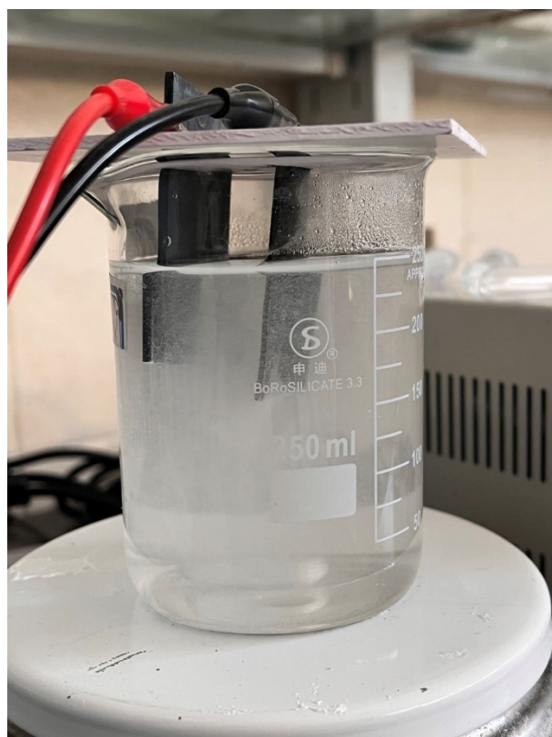
Fig. S3 Hydrogen evolution in high current reaction
