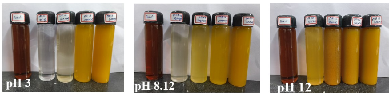
Fig S2 . Visual comparison of coir retting effluent before and after microwave-assisted Fenton treatment at different Fe 2+ concentrations (0.18 mM -8.96 mM) under various pH conditions. (a) Effluent color changes at pH 3 (b), at pH 8.12, and (C) pH 12
