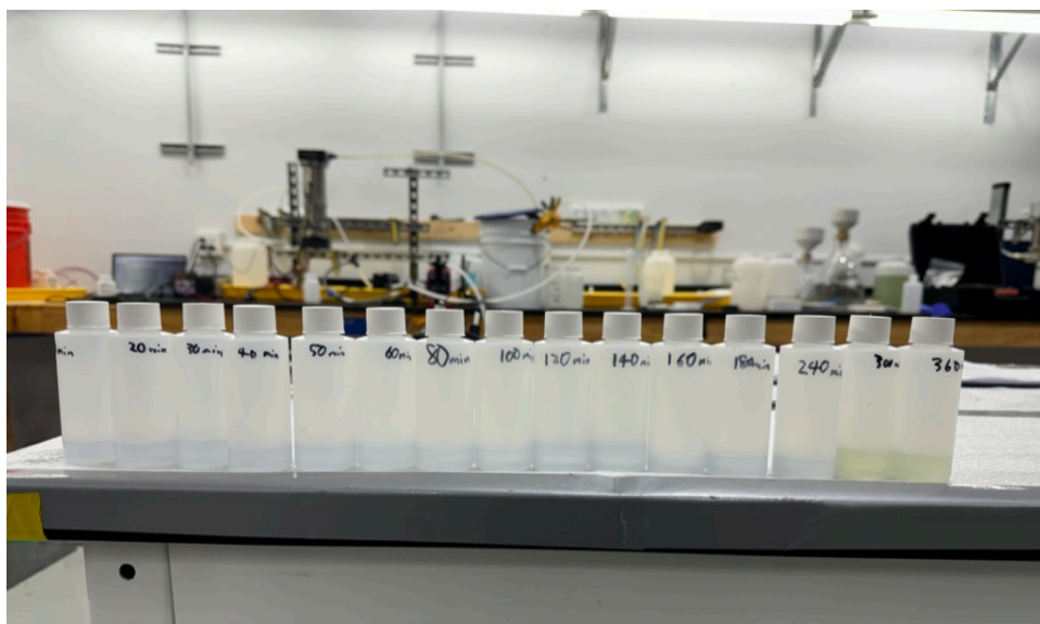
Figure S14: A series of hexavalent chromium samples taken over the course of a 6-hour reduction experiment using carbon-based anodes.
