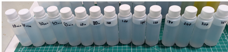
Figure S17: A series of hexavalent chromium samples taken over the course of a repeat 6-hour reduction experiment using mixed-metal oxide anodes.
