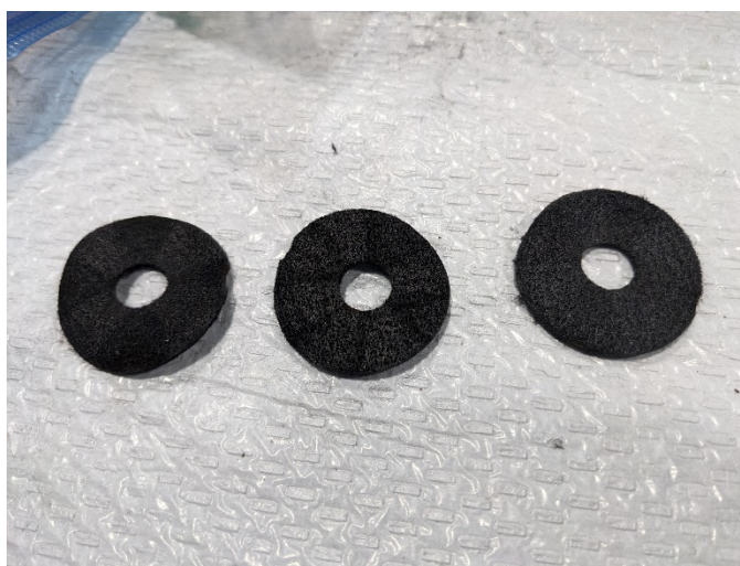
Figure S12: Used carbon cathodes from a deconstructed electrochemical cell used to reduce Cr(VI) in a pH 4 feed and an applied potential of 1.5 V.
