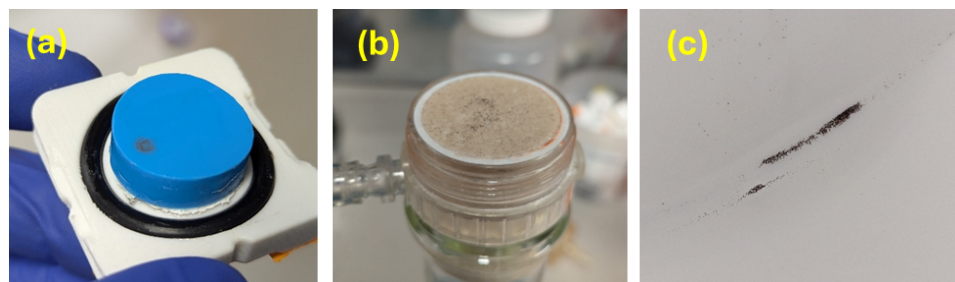
Figure S6 – Large loose iron oxide particles observed on a) pipe wall samples collected from the invert position of the pipes; b) filtered SSC samples collected from flushing phase of the experiments; and c) bottom of the bottles used to collect bulk water samples during the flushing phase of the experiment.
