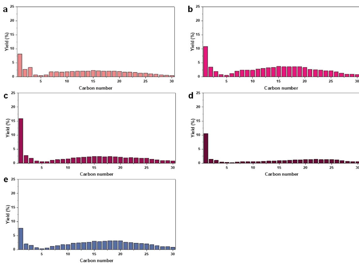
**Fig. S13** Product distributions of PE hydrogenolysis over Ru/Al<sub>2</sub>O<sub>3</sub> catalysts. (a) 0.5Ru/NA-Al<sub>2</sub>O<sub>3</sub>, (b) 1Ru/NA-Al<sub>2</sub>O<sub>3</sub>, (c) 5Ru/NA-Al<sub>2</sub>O<sub>3</sub>, (d) 8Ru/NA-Al<sub>2</sub>O<sub>3</sub> and (e) 1Ru/com-Al<sub>2</sub>O<sub>3</sub>. Reaction conditions: 3.0 g PE, 1 mg Ru, 250 °C, 40 bar H<sub>2</sub>, 2.5 h.
