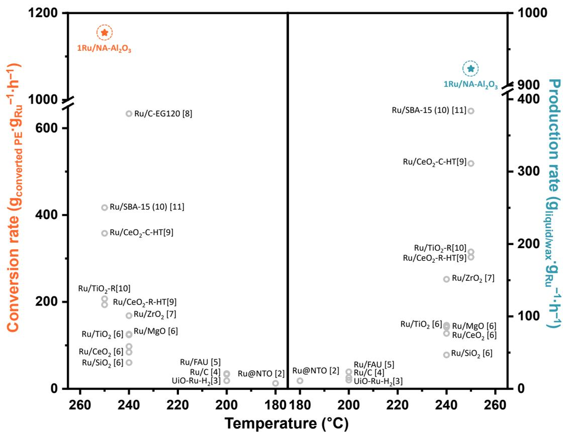
**Fig. S16** Performance comparison of this work with reported Ru-based catalysts in the hydrogenolysis of PE (Mw ~4,000, Mn ~1,700).<sup>2-11</sup>
