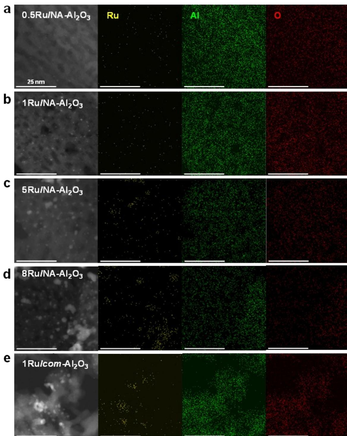
**Fig. S6** HAADF-STEM images and EDS elemental mappings of Ru/Al<sub>2</sub>O<sub>3</sub> catalysts. (a) 0.5Ru/NA-Al<sub>2</sub>O<sub>3</sub>, (b) 1Ru/NA-Al<sub>2</sub>O<sub>3</sub>, (c) 5Ru/NA-Al<sub>2</sub>O<sub>3</sub>, (d) 8Ru/NA-Al<sub>2</sub>O<sub>3</sub>, and (e) 1Ru/com-Al<sub>2</sub>O<sub>3</sub>.
