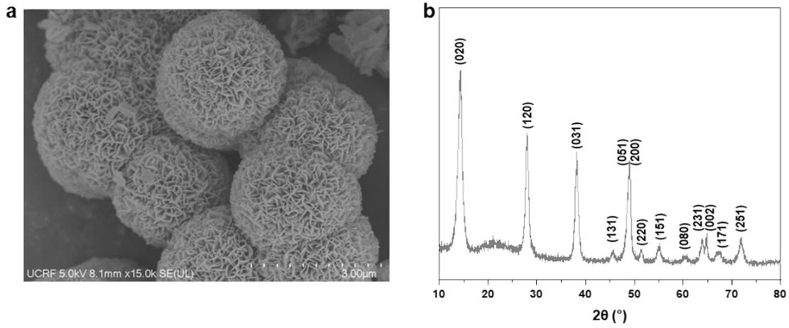
**Fig. S1** SEM image and XRD pattern. (a) SEM image and (b) XRD pattern (JCPDS 21-1307) of as-prepared NA-AlOOH.
