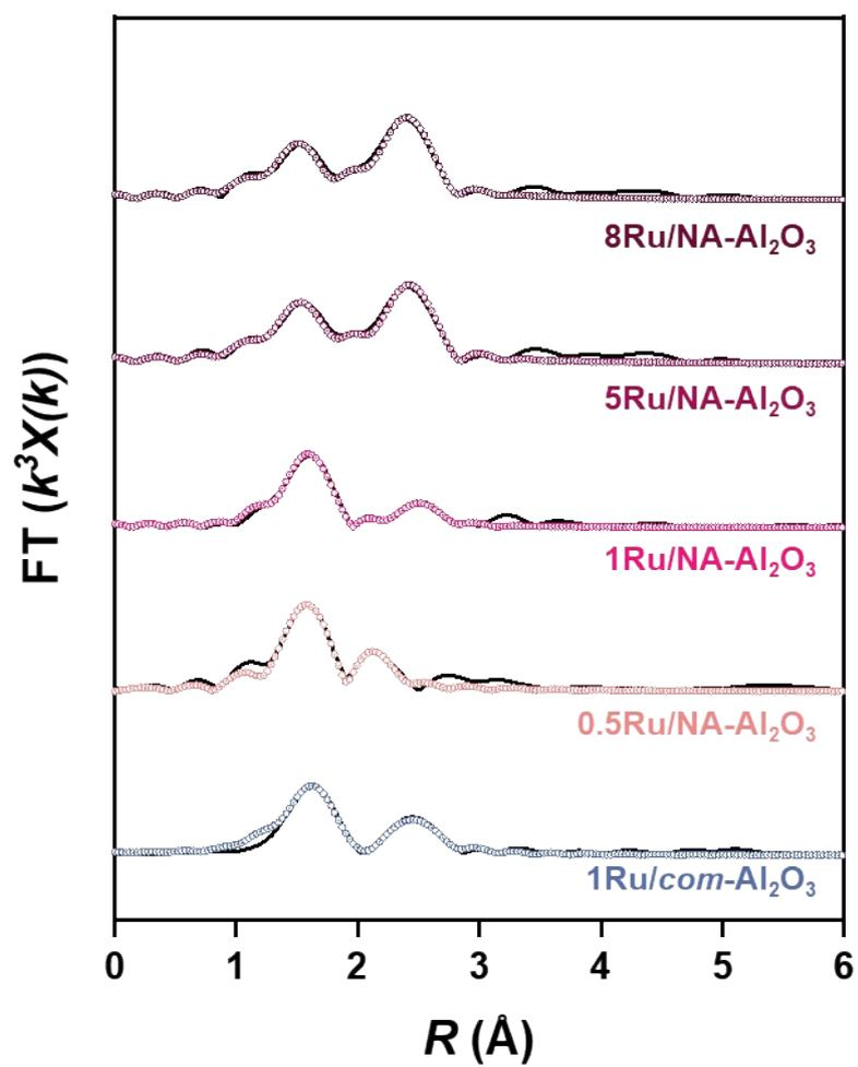
Fig. S11 Ru *K*-edge EXAFS *R*-space spectra and their fitting of Ru/Al<sub>2</sub>O<sub>3</sub> catalysts.
