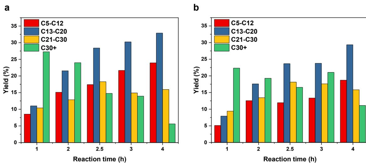
**Fig. S19** Time-dependent product distributions for (a) 1Ru/NA-Al<sub>2</sub>O<sub>3</sub> and (b) 1Ru/com-Al<sub>2</sub>O<sub>3</sub> catalysts. Reaction conditions: 3.0 g PE (M<sub>w</sub> ~4,000, M<sub>n</sub> ~1,700), 1 mg Ru, 250 °C, 40 bar H<sub>2</sub>.
