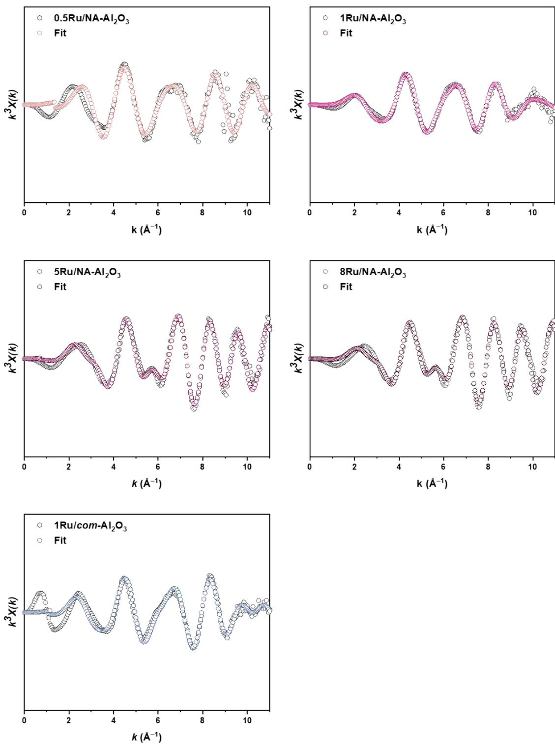
**Fig. S12** Ru *K*-edge EXAFS *k*-space spectra and their fitting of Ru/Al<sub>2</sub>O<sub>3</sub> catalysts.
