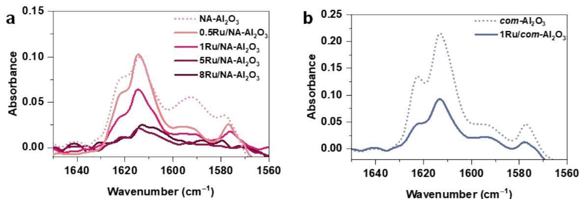
**Fig. S8** Pyridine-adsorbed DRIFT at 1650–1560  $\text{cm}^{-1}$  of Ru/ $\text{Al}_2\text{O}_3$  catalysts. (a)  $x\text{Ru}/\text{NA}-\text{Al}_2\text{O}_3$  and (b)  $1\text{Ru}/\text{com}-\text{Al}_2\text{O}_3$ .
