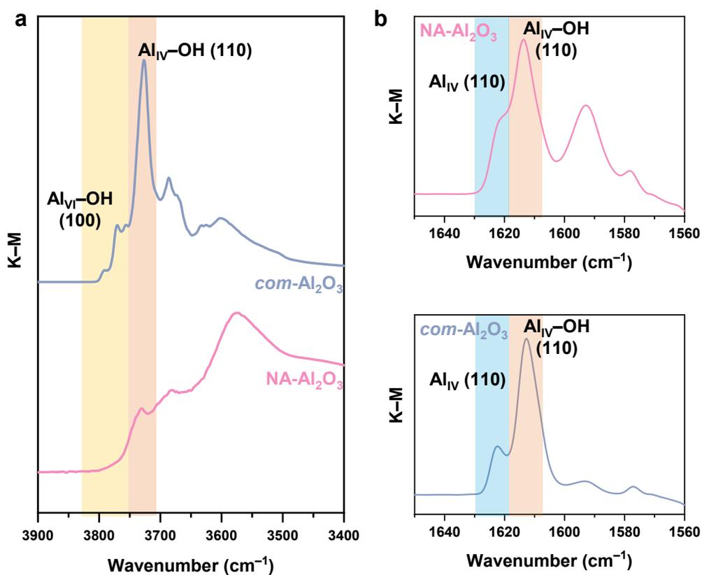
**Fig. S7** DRIFT spectra presented using the Kubelka–Munk (K–M) function. (a) *In situ* DRIFT spectra in OH stretching regions of NA-Al<sub>2</sub>O<sub>3</sub> and *com*-Al<sub>2</sub>O<sub>3</sub> at 25 °C. (b) Pyridine adsorbed DRIFT of NA-Al<sub>2</sub>O<sub>3</sub> and *com*-Al<sub>2</sub>O<sub>3</sub> at 100 °C (Normalized with the intensity of 1613 cm<sup>-1</sup>).
