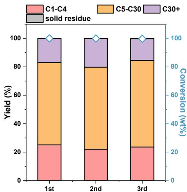
**Fig. S18** Reusability test of 1Ru/NA-Al<sub>2</sub>O<sub>3</sub> catalyst in PE hydrogenolysis. Reaction conditions: 3.0 g PE, 1 mg Ru, 280 °C, 40 bar H<sub>2</sub>, 1 h.
