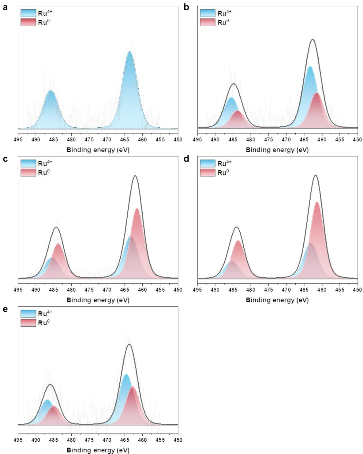
**Fig. S10** XPS profiles of Ru/Al<sub>2</sub>O<sub>3</sub> catalysts. (a) 0.5Ru/NA-Al<sub>2</sub>O<sub>3</sub>, (b) 1Ru/NA-Al<sub>2</sub>O<sub>3</sub>, (c) 5Ru/NA-Al<sub>2</sub>O<sub>3</sub>, (d) 8Ru/NA-Al<sub>2</sub>O<sub>3</sub>, and (e) 1Ru/com-Al<sub>2</sub>O<sub>3</sub>.
