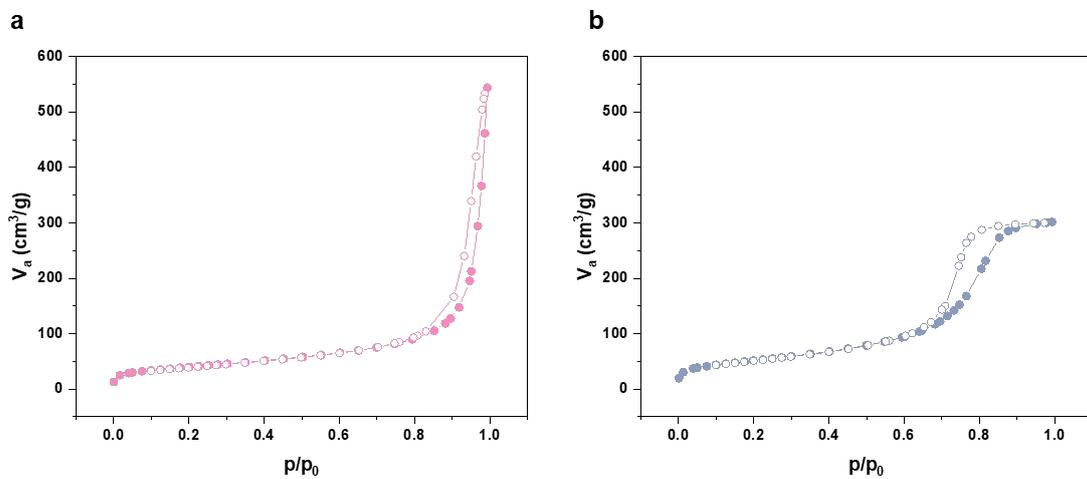
**Fig. S3** N<sub>2</sub> adsorption-desorption isotherms. (a) NA-Al<sub>2</sub>O<sub>3</sub> and (b) com-Al<sub>2</sub>O<sub>3</sub>.
