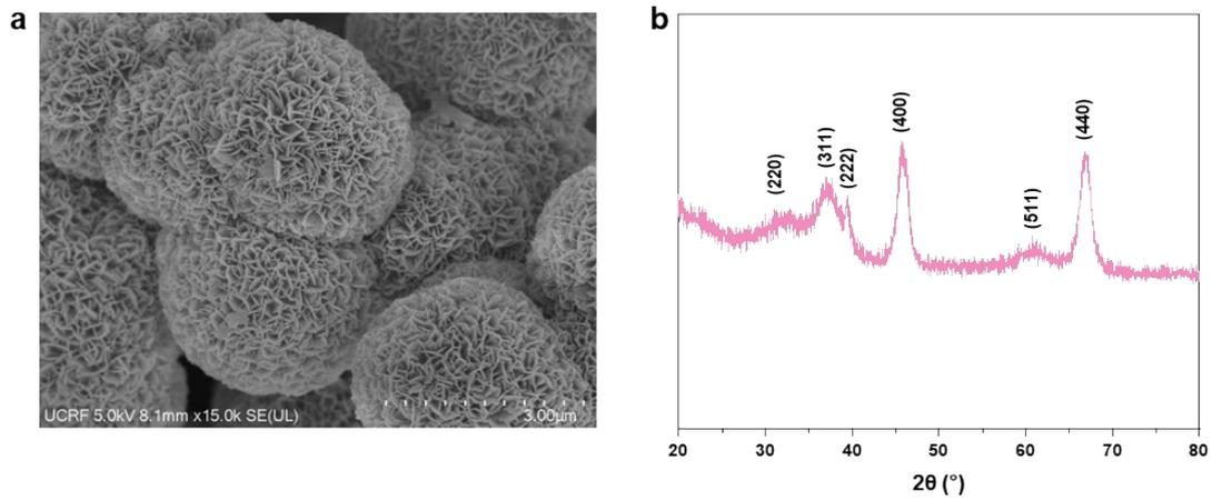
**Fig. S2** SEM image and XRD pattern. (a) SEM image and (b) XRD pattern (JCPDS 29-0063) of NA-Al<sub>2</sub>O<sub>3</sub>.
