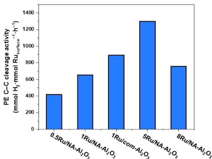
**Fig. S20** PE C–C bond cleavage activity of catalysts. Reaction conditions: 3.0 g PE ( $M_w \sim 4,000$ ,  $M_n \sim 1,700$ ), 1 mg Ru, 250 °C, 40 bar H<sub>2</sub>, and 2.5 h.
