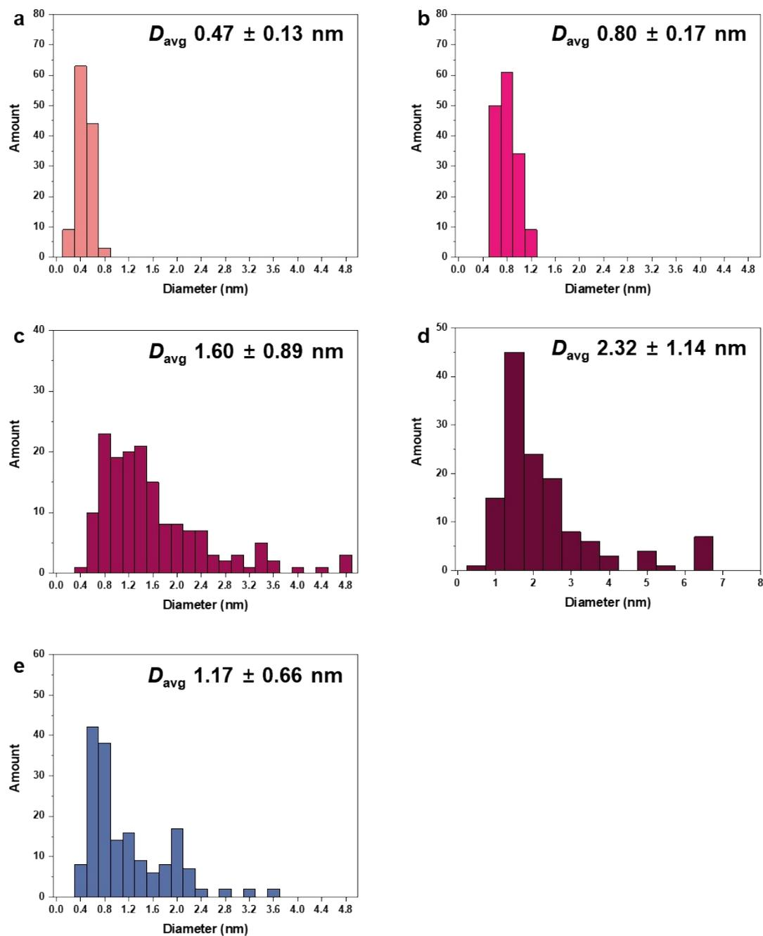
**Fig. S4** Particle size distributions of Ru/Al<sub>2</sub>O<sub>3</sub> catalysts. (a) 0.5Ru/NA-Al<sub>2</sub>O<sub>3</sub>, (b) 1Ru/NA-Al<sub>2</sub>O<sub>3</sub>, (c) 5Ru/NA-Al<sub>2</sub>O<sub>3</sub>, (d) 8Ru/NA-Al<sub>2</sub>O<sub>3</sub>, and (e) 1Ru/com-Al<sub>2</sub>O<sub>3</sub>.
