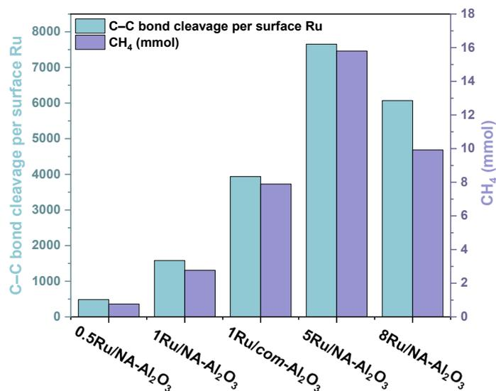
**Fig. S21** C–C bond cleavage per surface Ru and methane production under same reaction conditions in C<sub>18</sub>H<sub>38</sub> hydrogenolysis. Reaction conditions: 3.0 g C<sub>18</sub>H<sub>38</sub>, 0.5 mg Ru, 250 °C, 40 bar H<sub>2</sub>, 20 min.
