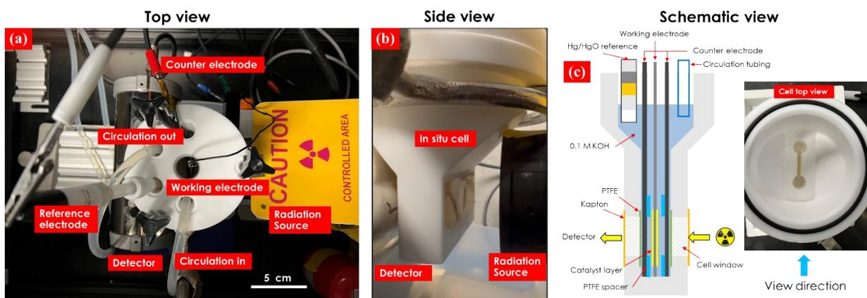
Figure S1. Photos and schematics of the experimental setup for *in situ* Mössbauer experiments.
