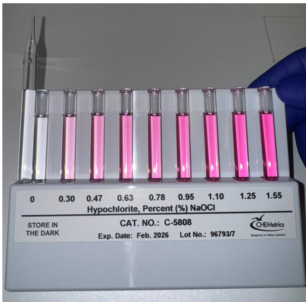
Fig. S17. Hypochlorite detection result for the electrolyte after 1.5 h seawater electrolysis at 500 \text{ mA cm}^{-2} .
