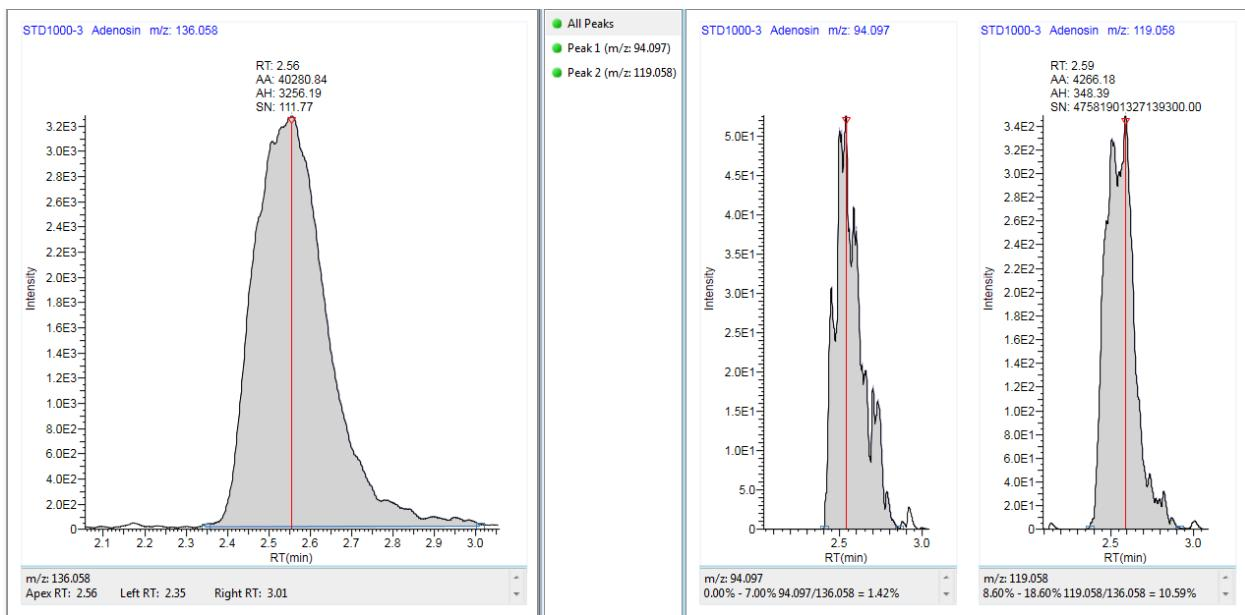
Figure S3. Representative chromatogram UHPLC-MS/MS of standard ADE at 100 ppb.
