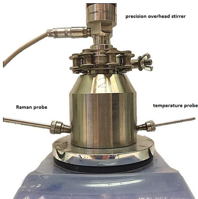
Figure S1: Experimental setup of the *in situ* Raman polymerization reactor.
