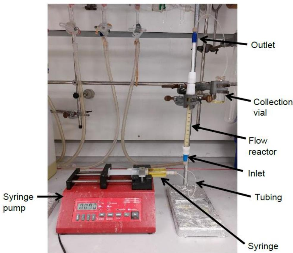
**Figure S1.** Continuous flow equipment set up with an AL-300 syringe pump fitted with a 20 mL plastic syringe and Omnifit<sup>®</sup> glass chromatography column.
