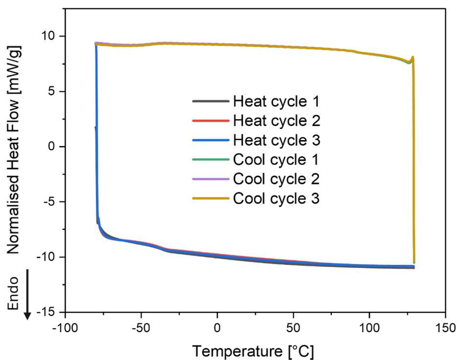
Figure S16. DSC thermogram of Resin A (57:31:12, EtLp<sub>1</sub>: HexLp<sub>2</sub>:LA) after post curing at 60 °C for 24 h (-80 – 130 °C, 10 °C×min<sup>-1</sup>, N<sub>2</sub>)
