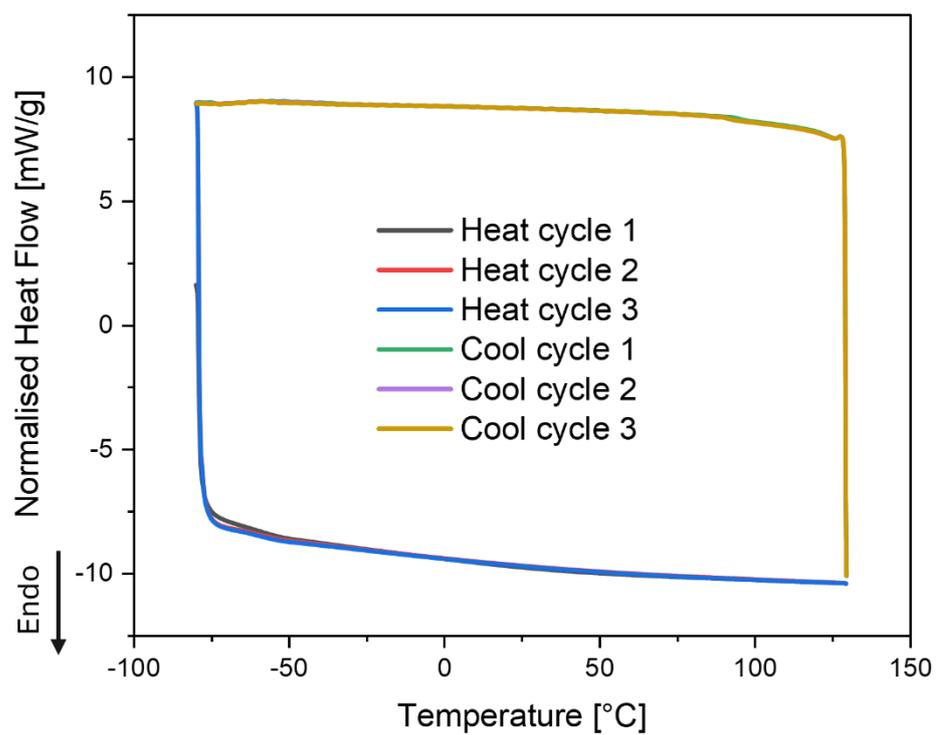
**Figure S17.** DSC thermogram of Resin B (66:18:16, EtLp<sub>1</sub>: HexLp<sub>2</sub>:LA) after post curing at 60 °C for 24 h (-80 – 130 °C, 10 °C×min<sup>-1</sup>, N<sub>2</sub>)
