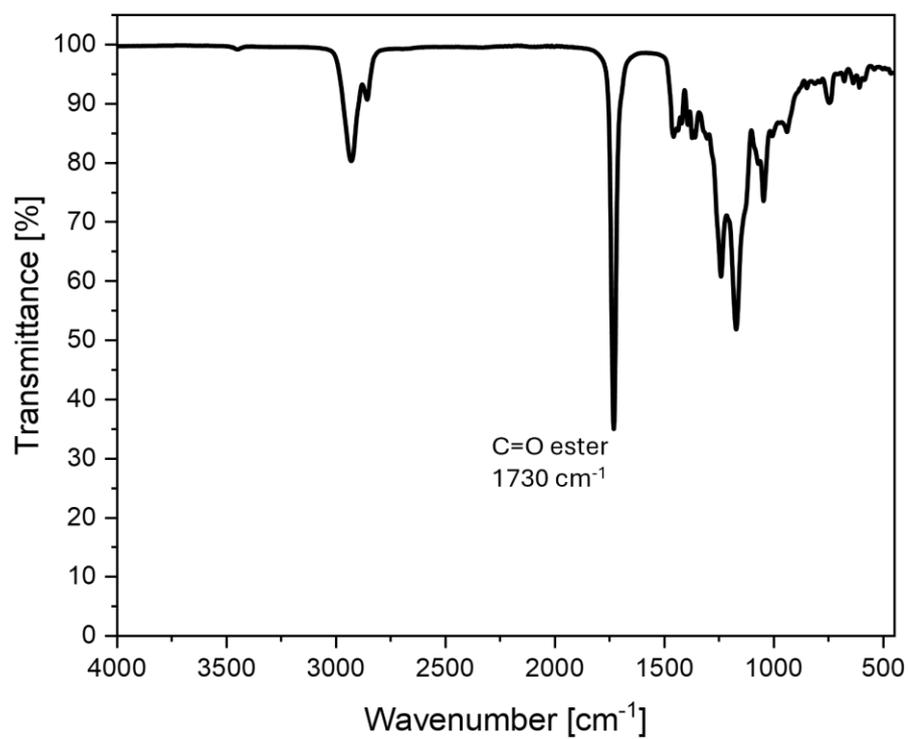
**Figure S11.** FT-IR spectrum of ButLp<sub>2</sub>.
