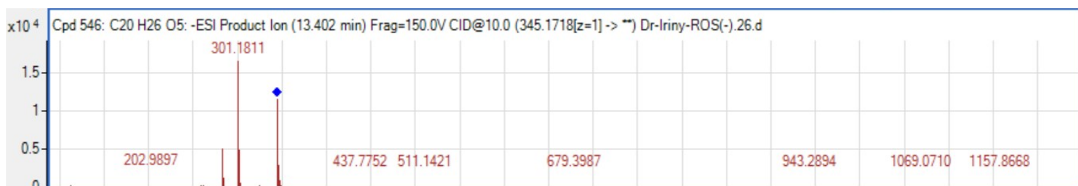
Fig. S2. ESI-MS/MS spectrum of peak (2) in the negative ion mode showing Rosmanol .
