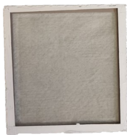
Figure SI-1. Photoanode composed of a \text{TiO}_2\text{:Nb} photocatalyst coated on a FTO glass substrate measuring 4.0\text{ cm} \times 4.3\text{ cm} . The white strip is the conductive silver paste and is 1\text{ cm} wide, resulting in a photocatalyst area of 3.0\text{ cm} \times 3.3\text{ cm} .
