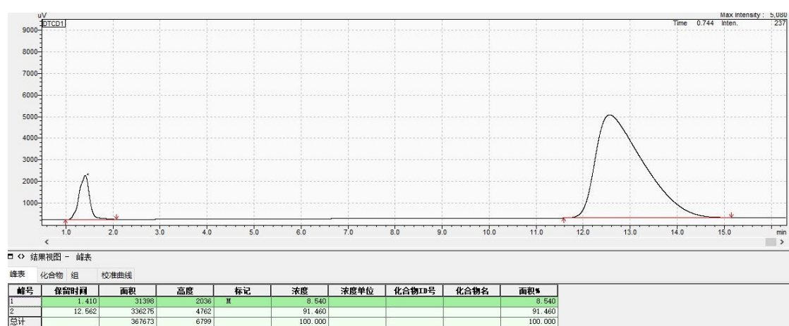
Figure S10 GC-TCD chromatogram of RWGR at 100 °C in the presence of TEA and LiCl
