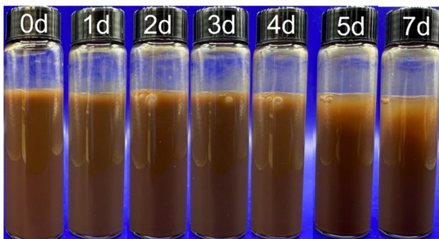
Fig. S17. Long-term stability of aminated LNP in a size range of 339 \pm 72 nm derived from the bamboo-biomass
